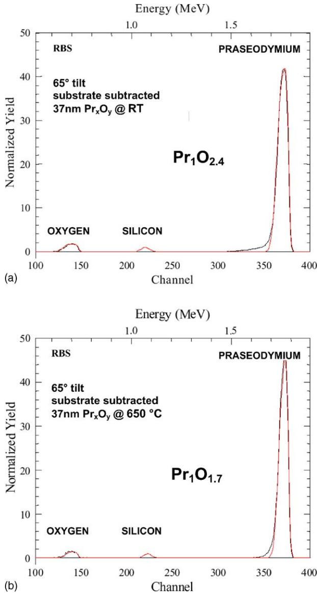
Fig. 5. The energy distribution of backscattered  $^4\text{He}^+$  ions from two samples with same film thickness of 37 nm. The  $\text{Pr}_x\text{O}_y$  layers were grown at RT (upper graph) and at  $650^\circ\text{C}$  (bottom graph), respectively. The peaks, corresponding to oxygen, silicon, and praseodymium are labelled. The element ratio Pr:O is indicated.
