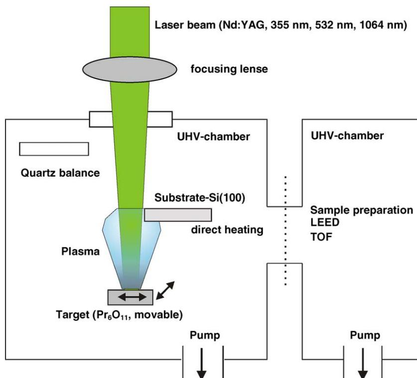
Fig. 1. A schematic diagram of the experimental arrangement for the growth of thin  $\text{Pr}_x\text{O}_y$  films on p-Si(100) substrates by pulsed laser deposition. The  $\text{Pr}_6\text{O}_{11}$  target material was placed in a Ta-holder which was moved continuously during the whole growth procedure.
