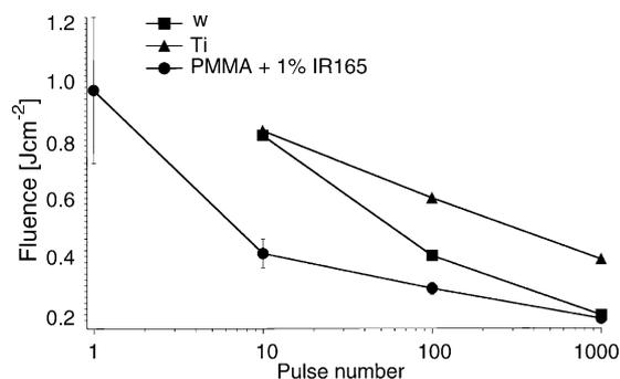
Fig. 6. Ablation threshold fluence for tungsten (■), titanium (▲) and doped PMMA (●) [5] vs. pulse number for ns laser treatment.
