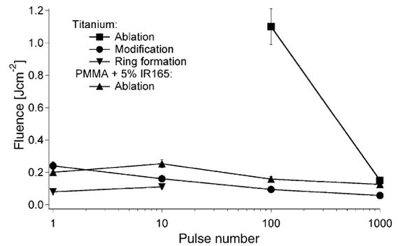
Fig. 4. Ablation threshold fluence for titanium (■) and doped PMMA (▲) [5] vs. pulse number for fs laser exposure. The onset fluence of the surface modification (●) and the ring formation (▼) for titanium are also shown.
