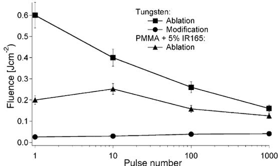
Fig. 1. Ablation threshold fluence for tungsten (■) and doped PMMA (▲) [5] vs. pulse number for fs laser irradiation. Also the onset fluence of the surface modification for tungsten is shown (●).
