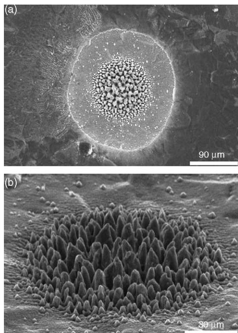
Fig. 3. SEM picture of titanium after fs laser irradiation with 100 pulses and  $1.7 \text{ J cm}^{-2}$  at 1 kHz as overview (a) and detailed view of the columnar surface modification (b).
