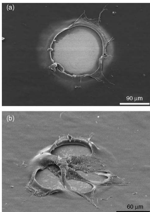
Fig. 7. SEM picture of the ablation spot of doped PMMA on tungsten after fs laser irradiation with two pulses  $1.87 \text{ J cm}^{-2}$  (a) and  $0.45 \text{ J cm}^{-2}$  (b).
