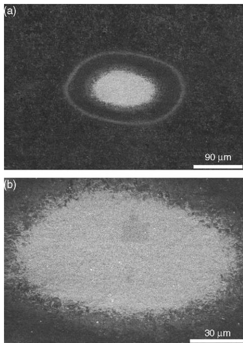
Fig. 2. Scanning electron microscope (SEM) picture of tungsten after fs laser treatment with 100 pulses and  $1.6 \text{ J cm}^{-2}$  at 1 kHz as overview (a) and detailed view of the “white” surface modification (b).
