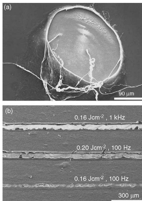
Fig. 8. SEM picture of the ablation spot of doped PMMA on tungsten after ns laser irradiation with 100 pulses and  $1.95 \text{ J cm}^{-2}$  (a) and in (b) the influence of the pulse repetition rate and the irradiation fluence for fs laser irradiation of doped PMMA on tungsten is shown.
