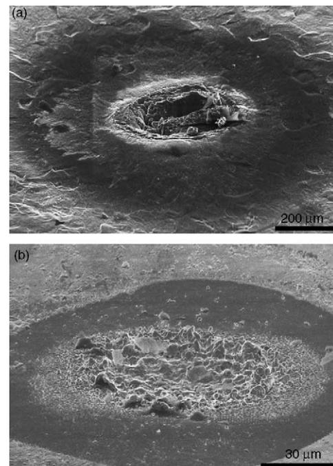
Fig. 5. Scanning electron microscope (SEM) picture of titanium after ns laser irradiation with 1000 pulses and  $1 \text{ J cm}^{-2}$  at 10 Hz (a) and SEM picture of the ablation spot of tungsten after ns laser irradiation with 100 pulses and  $1.3 \text{ J cm}^{-2}$  at 10 Hz (b).
