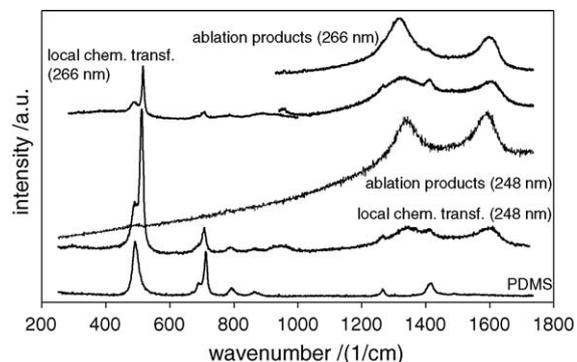
Fig. 4. Representative Raman spectra of native PDMS, the local chemical transformations and the ablation products after irradiation with the Nd:YAG (266 nm) and the KrF<sup>\*</sup>-excimer laser (248 nm).
