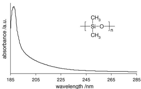
Fig. 1. UV absorption spectra of PDMS.
