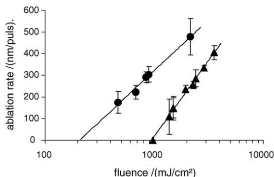
Fig. 2. Plot of etch depth per pulse vs. fluence: (▲) 248 nm and (●) 266 nm.
