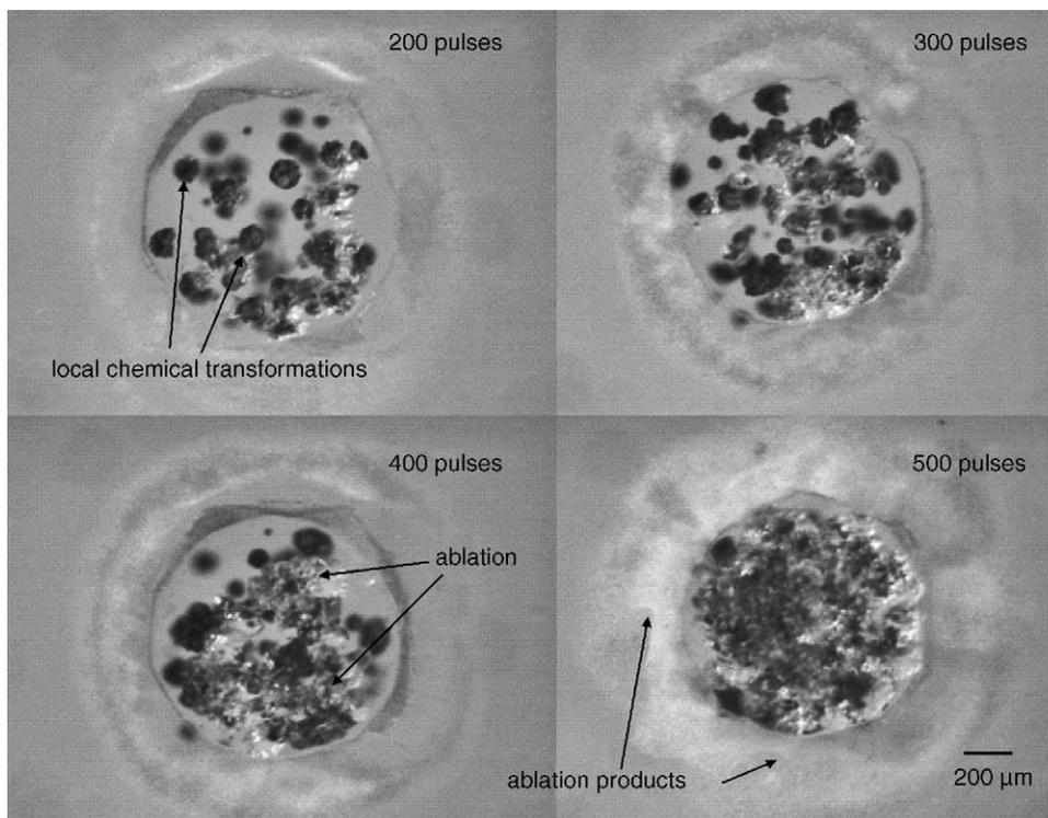
Fig. 3. Optical microscope photographs of irradiated PDMS samples (KrF<sup>\*</sup>-excimer laser, 248 nm,  $1 \text{ J cm}^{-2}$ , 200–500 pulses). The microscope was focused onto the surface. The local chemical transformations located below the surface appear less sharp. Areas of ablation and the ablation products are clearly visible.
