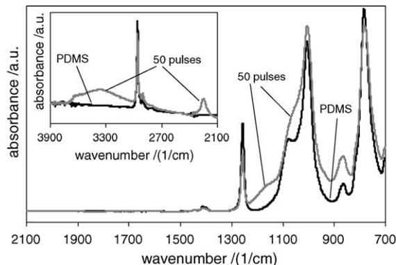
Fig. 5. ATR-FTIR spectra of native PDMS and the ablation products after irradiation with the KrF<sup>\*</sup>-excimer laser ( $248\text{ nm}$ ,  $4.8\text{ J cm}^{-2}$ , 50 pulses).
