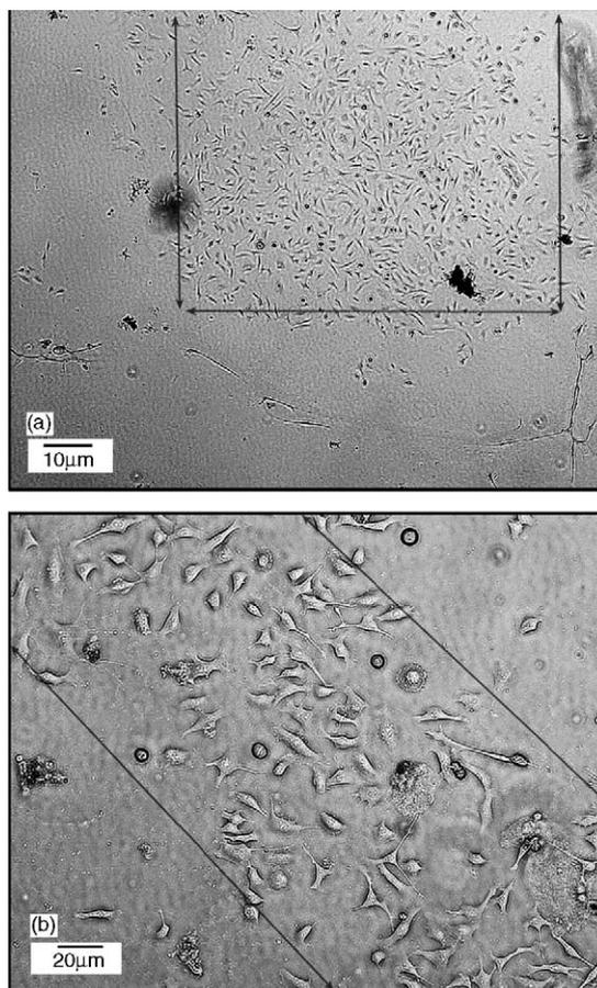
Fig. 4. (a) Optical micrograph of MAPLE DW transferred B35 neuroblasts into pre-defined patterns such as a box-like pattern. Scale equals 100  $\mu$ m. (b) Line-like cell patterns. Scale equals 20  $\mu$ m. Arrows are drawn to guide the eye.
