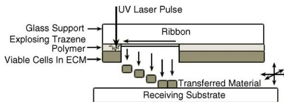
Fig. 2. Schematic of MAPLE DW, a laser-based technique for patterning organic, inorganic and living materials. A novel variation in using absorbing layer such as triazene polymer allows a softer transfer.
