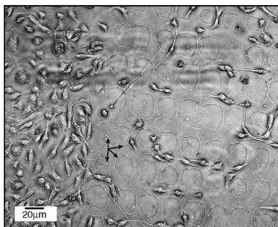
Fig. 3. Optical micrograph of the ribbon used for MAPLE DW transfer of B35 neuroblasts. Arrows indicate circular regions of desorbed polymer due to the absorption of incident light causing forward transfer of viable cells. Scale equals 20  $\mu$ m.
