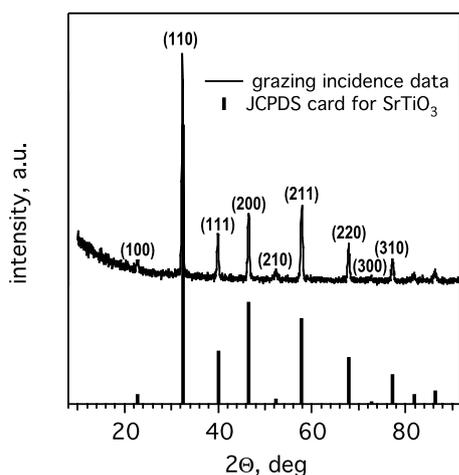
**Fig. 3** Typical grazing incidence diffraction pattern of the N-doped  $\text{SrTiO}_3$  film (deposited using  $\text{N}_2$  RF-plasma at a flow rate of 100 sccm and a RF-power of 100 W). All observed reflections are in agreement with those of  $\text{SrTiO}_3$ , confirming the perovskite-type phase purity
