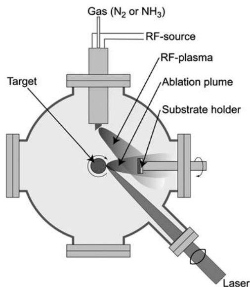
**Fig. 1** Experimental setup for the RF-plasma assisted pulsed laser deposition. A continuous plasma beam (RF-plasma) generated by the RF-discharge is directed to the substrate, which gives additional control over the anionic composition of the film grown by PLD
