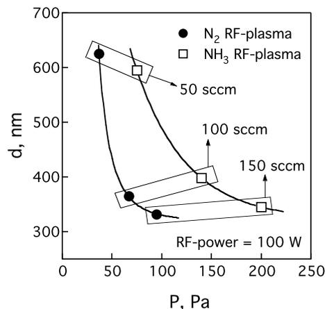
**Fig. 4** Thickness of the  $\text{SrTiO}_3$ -based films deposited by RF-plasma assisted PLD at different flow rates as a function of the deposition pressure. Solid lines are plotted for visual guidance only
