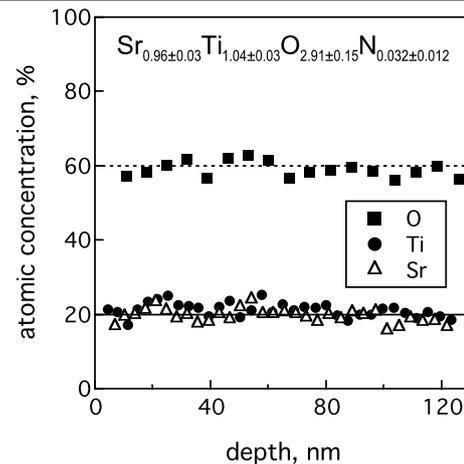
**Fig. 5** ERDA depth-profile of the chemical composition of the film deposited using the N<sub>2</sub> RF-plasma at a flow rate of 100 sccm and a RF-power of 100 W
