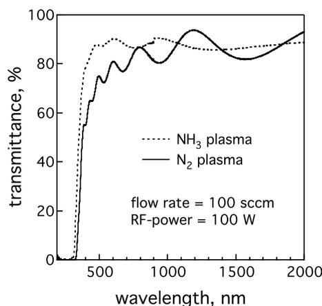
**Fig. 7** Typical transmittance spectra of the studied  $SrTiO_3$ -based films. N-doped films deposited in  $N_2$  RF-plasma reveal an absorption shoulder in the visible range of wavelength ( $\sim 400$ – $600$  nm), which is associated with nitrogen incorporation into the perovskite-type crystal lattice. The oscillations above 500 nm are due to interference phenomena
