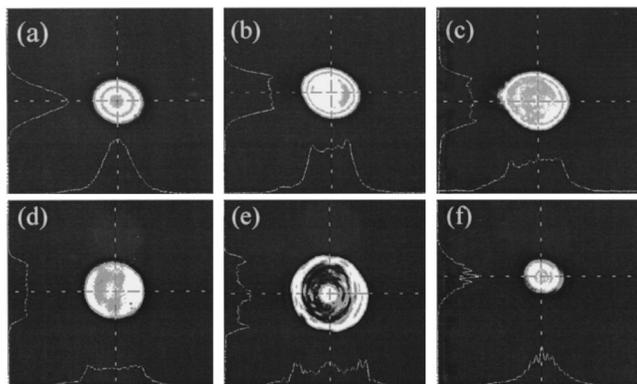
FIG. 2. Images of the transmitted laser beam: (a)–(c) 150  $\mu\text{m}$  thick BK-7 cover slip: (a) 40  $\mu\text{J}$ , (b) 184  $\mu\text{J}$ , (c) 395  $\mu\text{J}$  incident pulse energy; (d)–(e) 1 mm sapphire: (d) 19  $\mu\text{J}$ , (e) 40  $\mu\text{J}$  incident pulse energy; (f) 1 mm BK-7: 7.3  $\mu\text{J}$  incident pulse energy. These are gray-scale representations of false color images.
