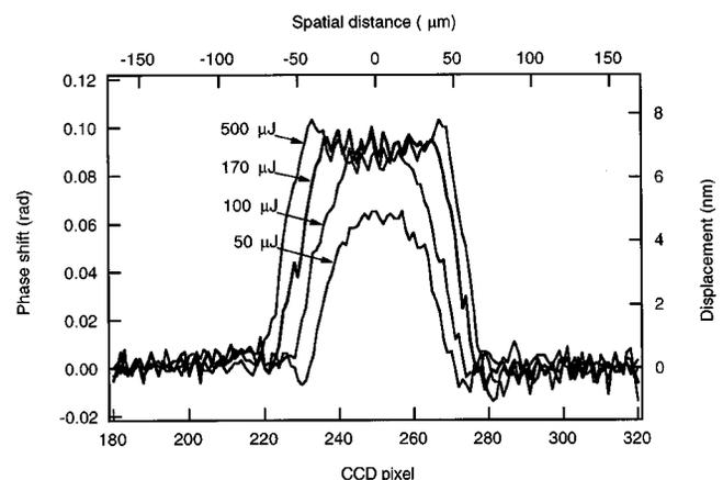
FIG. 1. Shock profile at several incident laser energies for a 1  $\mu\text{m}$  Al film deposited on a 150  $\mu\text{m}$  thick borosilicate glass microscope cover slip.
