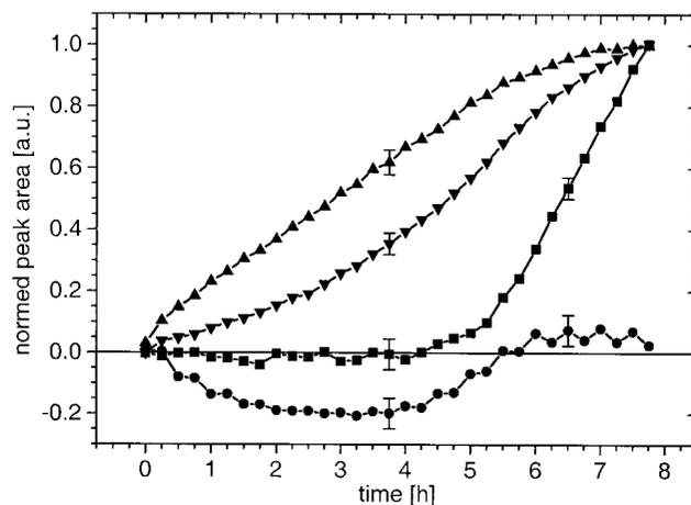
FIG. 3. Changes of the normalized peak area of the bands at  $725 \text{ cm}^{-1}$  [(▲) the out-of-plane bending of the imide ring], at  $3060 \text{ cm}^{-1}$  [(▼) C–H stretching vibrations of the aromatic ring], at  $1750 \text{ cm}^{-1}$  [(■) imide and amide C=O stretching vibration], and at  $2220 \text{ cm}^{-1}$  [(●) C=N stretching vibration]. The experiment was performed at 812 K using a total flow of  $50 \text{ mL}_N \text{ min}^{-1}$  of compressed air.
