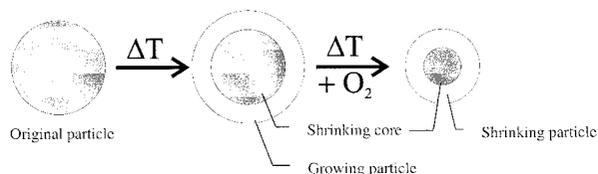
Fig. 6. Suggested decomposition scheme: shrinking particle with a shrinking core. The pyrolysis of the core has an Arrhenius activation energy of  $E_A = 162 \pm 19 \text{ kJ mol}^{-1}$  (imide rings), and the pyrolysis of the residual particle one of  $E_A = 212 \pm 37 \text{ kJ mol}^{-1}$  (aromatic rings).
