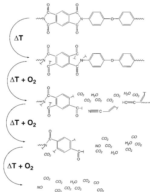
FIG. 4. Suggested scheme of the thermal decomposition of Kapton, including various intermediates, assuming a total oxidation of the carbon.  $\perp$  indicates a broken bond; information on the nature (radicalic, ionic, terminated) is not available from the present experiments.
